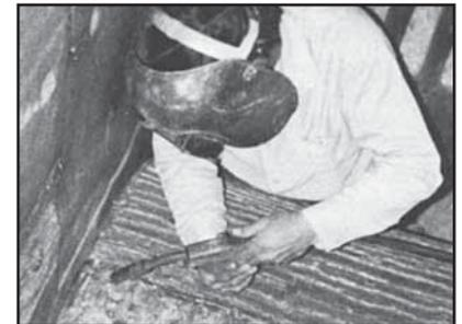
Crusher Roll hardfaced with 2820-MCO after application of Postalloy 2865-FCO
