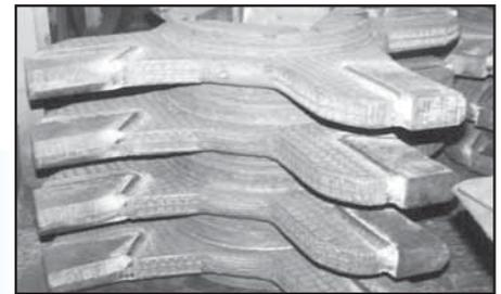
Sinter Breaker overlayed with 2834-MCO
