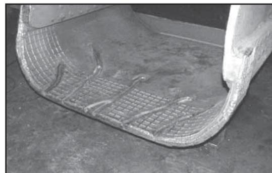
Bucket prepared for repair welding with 3044-FCG.
